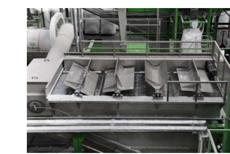
Sink/Float Tank for HDPE plastic recovery (Source: Summit Systems Ltd)
