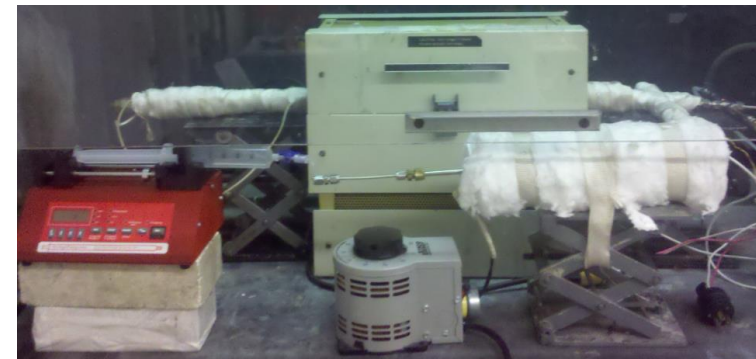
Isothermal testing, under synthetic WTE flue gas
