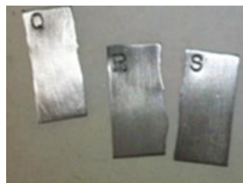
Coupons cut from SH alloys, 3.2 cm 2 area
