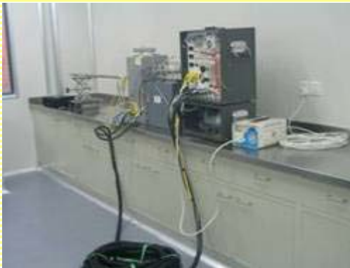
dioxin source sampling system USEPA M23
