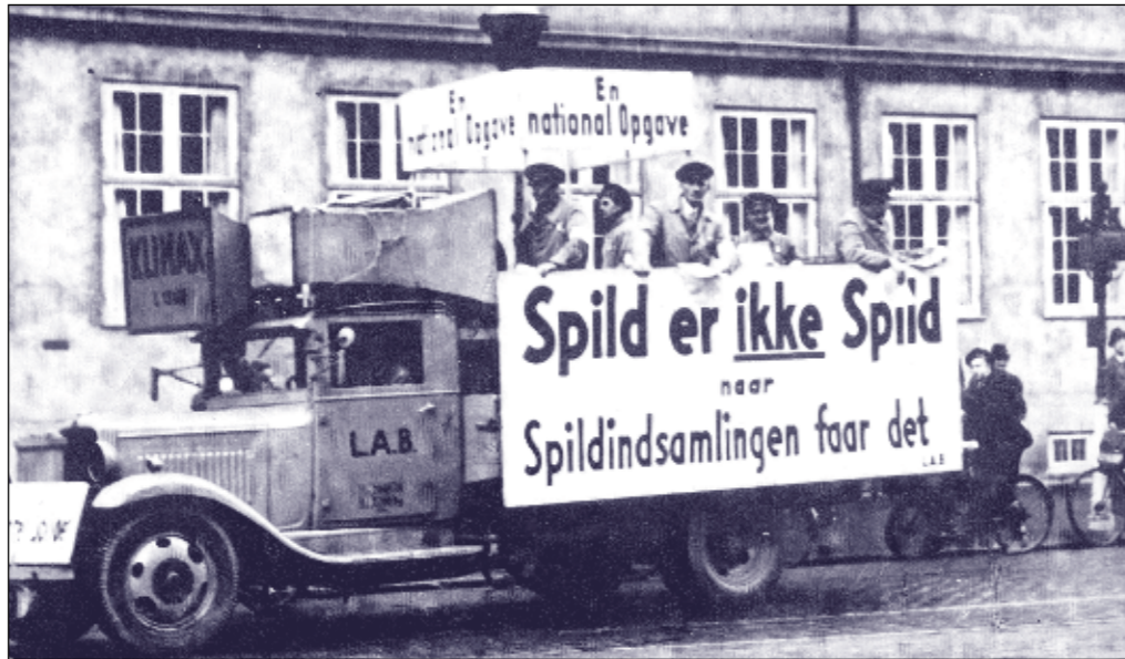
During the German occupation waste salvaging was so well organised that there was practically no incinerable waste left for the waste incineration plants. The sign on the vehicle in the photo says: 'Waste is not a waste when the refuse salvagers get it'. Also note the gas generator in the front of the car.
