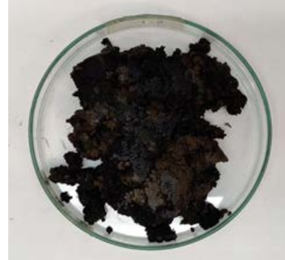
Dewatered sewage sludge from Kranji WRP (K-DWS)
