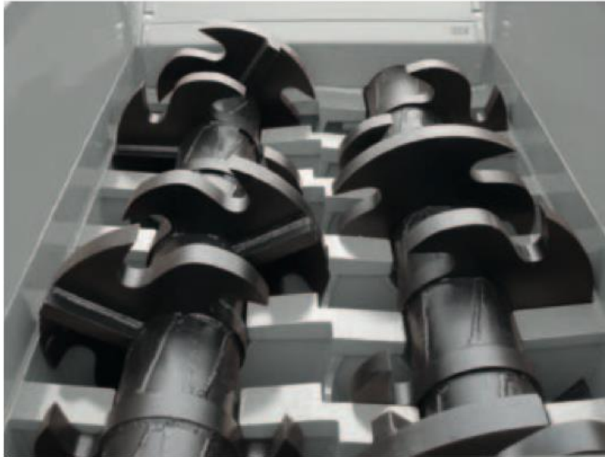
Figure 30 - Metso LSHT shredders for MSW. Image from metso.com
