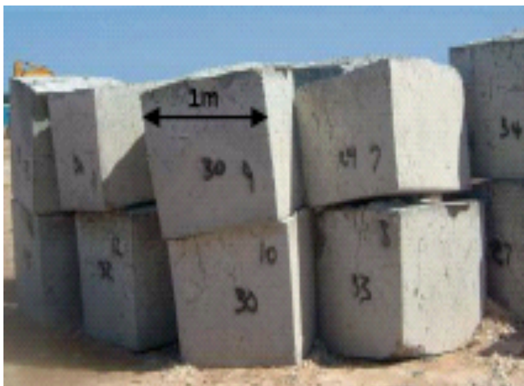
Figure 36 Concrete blocks made from WTE ash used for shore protection and land reclamation 35
