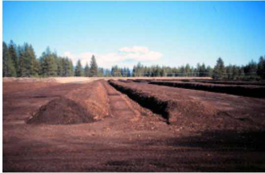
Figure 75: Windrow composting. (Washington State University, 2000).
