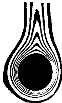
Figure 12.11. Interference photograph showing variation of thickness of natural convection boundary layer around a horizontal heated tube.
