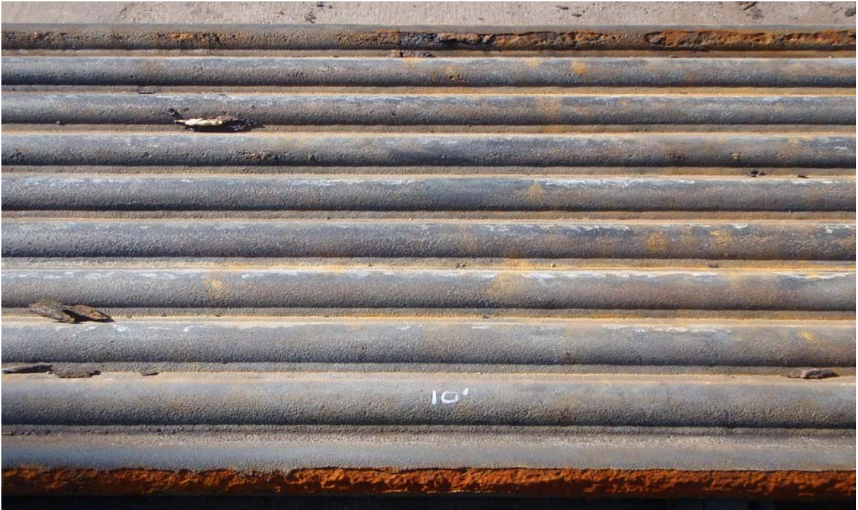
Figure 12. AmStar Panel 3-4 after 2 years of operation at top 10' from Roof (lead tube at the front).
