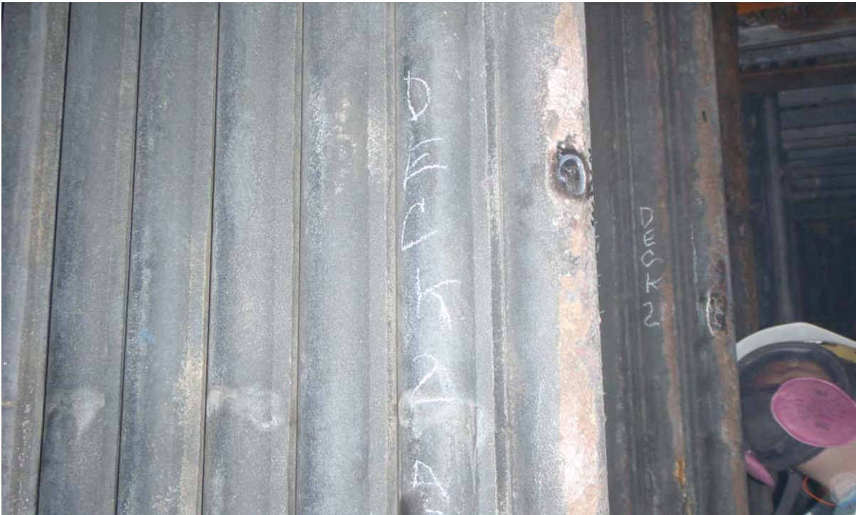
Figure 10. AmStar Panel 3-4 (left) and Coating Y Panel 3-5 (right) after one year of operation.
