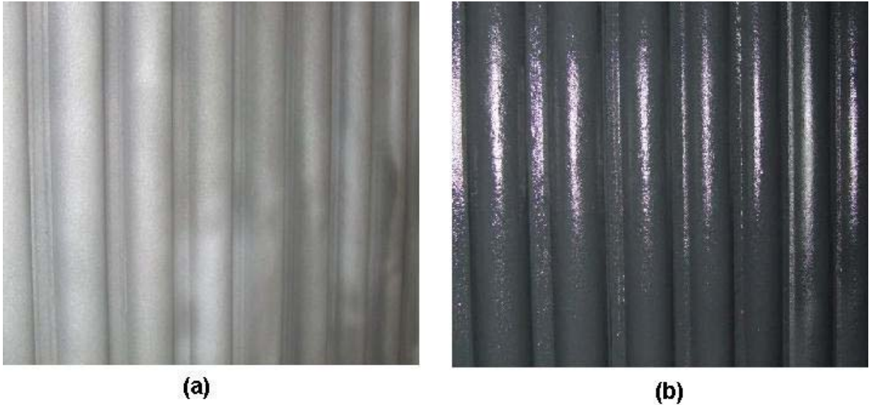
Figure 2. The cladding as sprayed (a), and after application of the surface passivator (b).
