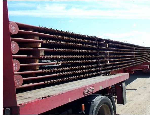
Figure 9a – platen superheaters EfW plant Naples/Italy, transport to site
