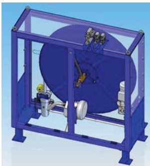
Figure 5 Shower Cleaning System as a stand-alone module
