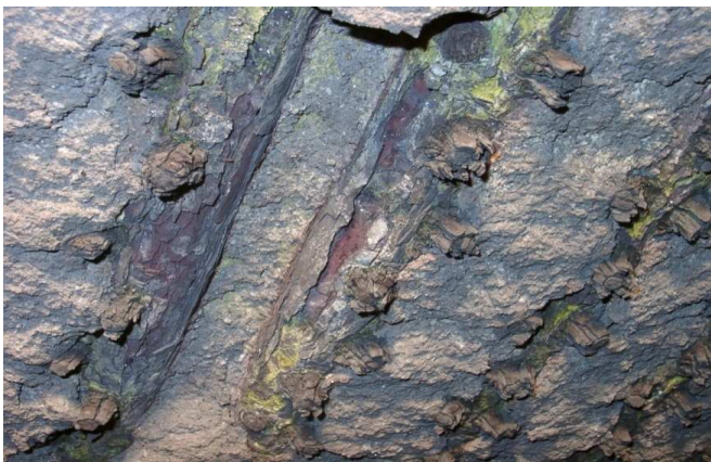
Figure 16: Tube wall with refractory lining out of SiC mixes after approx. 2 years of operation
