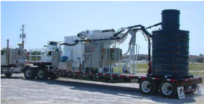
Figure 1: Furnace portion of the Transportable Waste-to-Energy System
