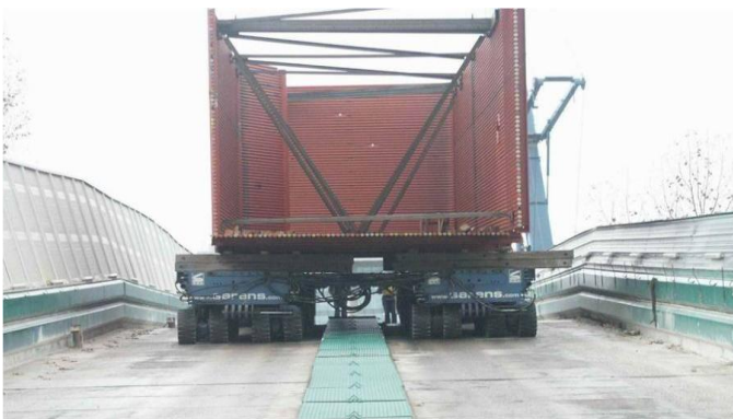
Figure 7, boiler module being transported
