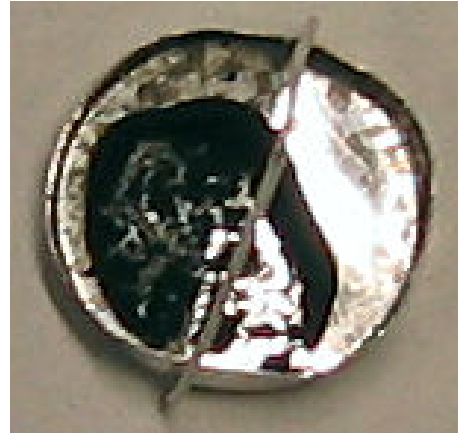
Figure 4. Smaller char film from 20% CO 2 spruce steam gasification
