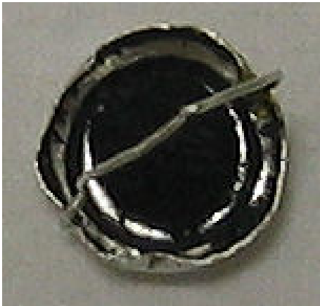
Figure 5. Large black char residue from 0% CO 2 walnut shells steam gasification
