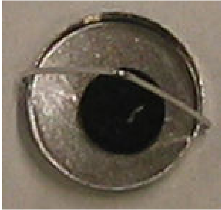
Figure 3. Large black char residue from 10% CO 2 spruce steam gasification
