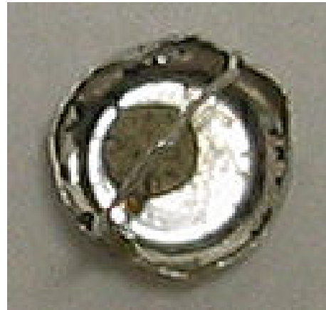
Figure 6. Small light mineral residue pancake from 30% CO 2 walnut shells steam gasification
