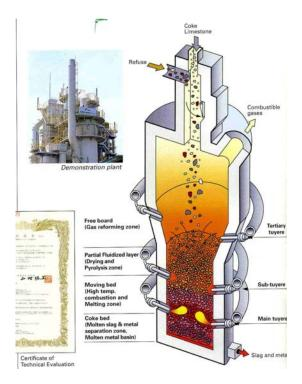
Figure 3. The JFE Direct Smelting Process
