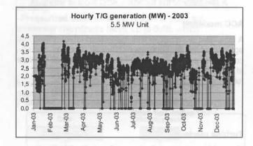
Fig. 1 2003 Power Generation from the 5.5 MW unit
