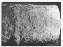
FIGURE 1 - Close-up of rough, wasted surface covered with friable corrosion product layers.
