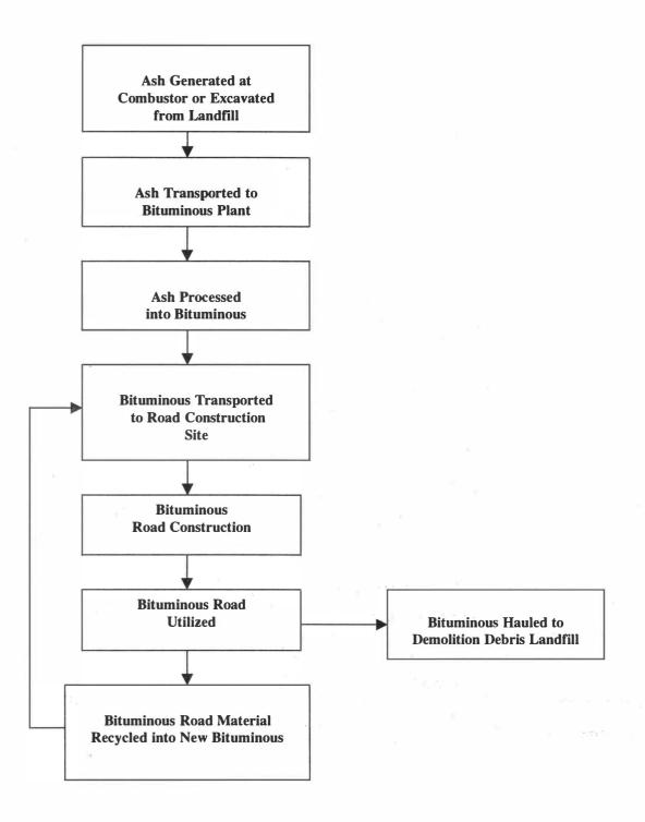
FIGURE 1 ASH PRODUCT FLOW DIAGRAM
