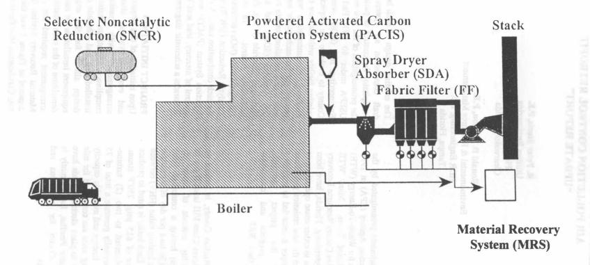
Figure 1 - APC SYSTEM SCHEMATIC
