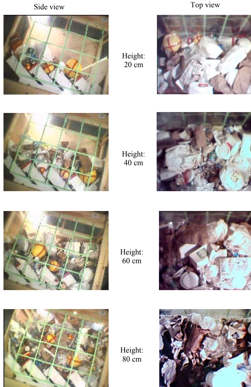
Figure 3-9: Side views and top views of NYC-MSW beds with 20, 40, 60, and 80 cm heights and angles of chamber bed decline: 15 degree
