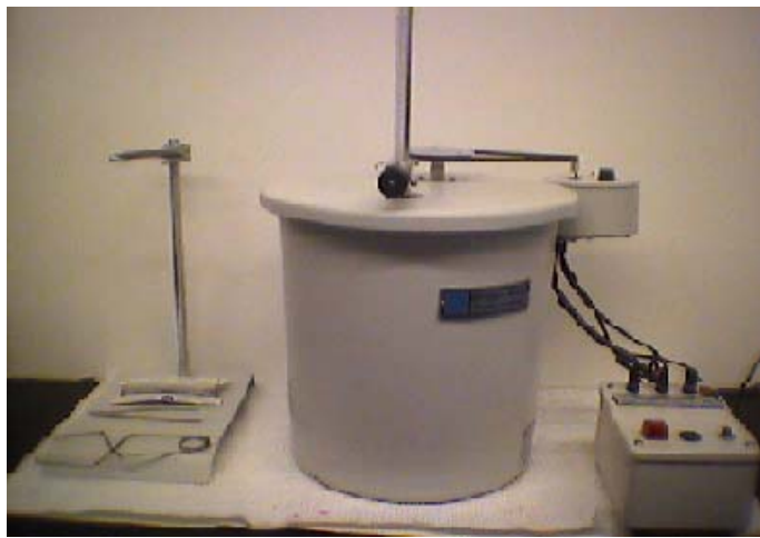
Figure 2: Parr Bomb Calorimeter used in analysis
