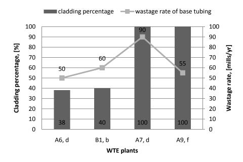
Figure 3-2 Waterwall cladding percentage and wastages rate of the base tubing
