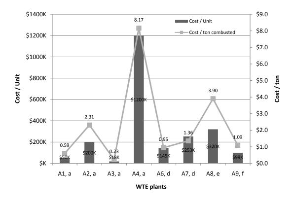
Figure 3-18 Yearly operating cost due to corrosion
