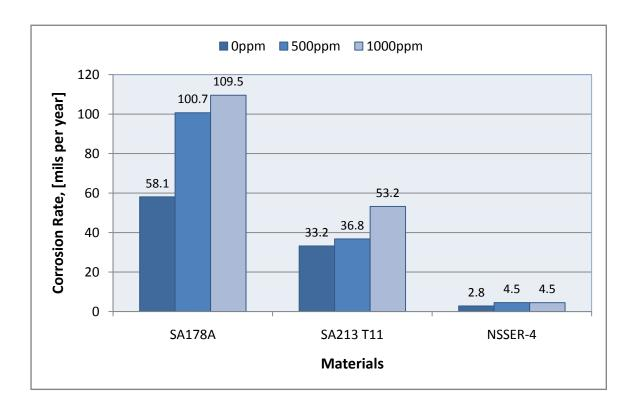
Figure 5-38 The comparison of corrosion rates of three materials
