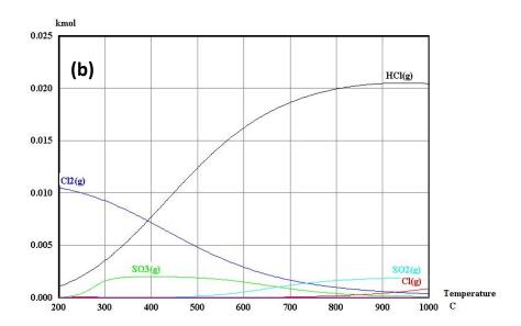
Figure 5-14 The concentrations of the major corrosive gases within the testing temperature range (a) without HCl gas and (b) with 1000ppm HCl gas
