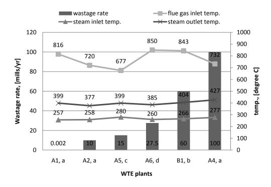
Figure 3-17 Superheater wastage rate, flue gas inlet, steam inlet and outlet temperature
