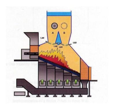
Figure 2-3 Schematic diagram of the Seghers Boiler Prism [6]
