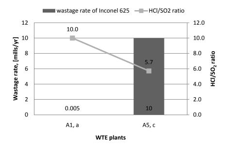
Figure 3-11 Wastage rates of Inconel 625 and HCI/SO<sub>2</sub> ratio
