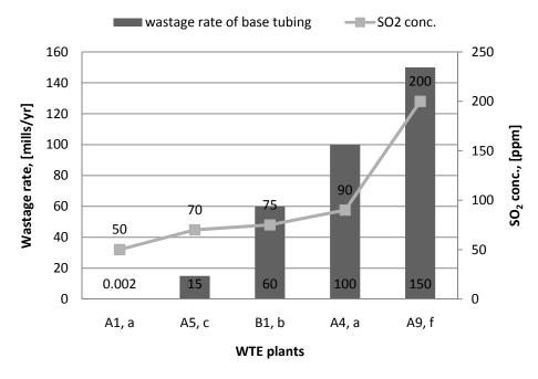
Figure 3-15 Wastage rates of superheater base tubing and  $SO_2$  conc. before in process gas
