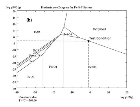
Figure 5-19 Stability diagrams of the system at  $560^{\circ}$ C (with 1000ppm HCl) (a) Fe-O<sub>2</sub>-Cl<sub>2</sub> and (b) Fe-O<sub>2</sub>-SO<sub>2</sub> [40]
