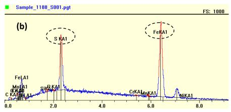
Figure 5-17 (a) SEM images of the scale/metal interface after removal of scale (without HCl), and (b) Elemental analysis of the scale/metal interface
