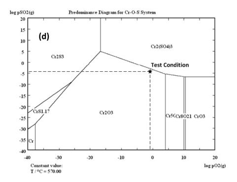
Figure 5-27 Stability diagrams of the system at  $570^{\circ}$ C (with 1000ppm HCl) (a) Fe-O<sub>2</sub>-Cl<sub>2</sub>, (b) Fe-O<sub>2</sub>-SO<sub>2</sub>, (c) Cr-O<sub>2</sub>-Cl<sub>2</sub>, and (d) Cr-O<sub>2</sub>-SO<sub>2</sub> [40]
