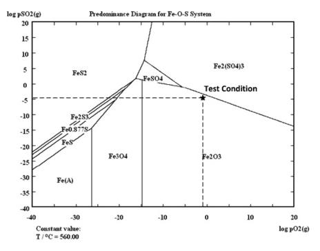
Figure 5-16 Stability diagram of the Fe-SO<sub>2</sub>-O<sub>2</sub> system at 560°C (without HCI) [40]
