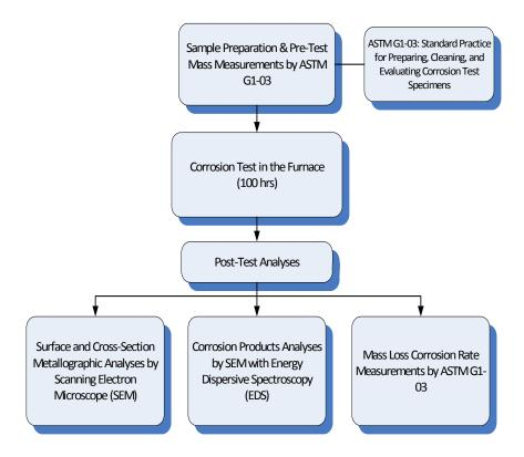
Figure 4-1 Experimental procedures of the corrosion test
