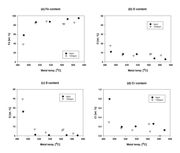
Figure 5-29 Elemental analysis of the scales' surfaces; (a) Fe, (b) O, (c) S and (d) Cr
