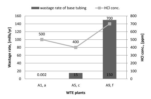
Figure 3-14 Wastage rates of superheater base tubing and HCl conc. before in process gas
