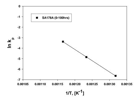
Figure 5-3 Temperature dependence of oxidation rate constant of SA178A within the 100-hour test
