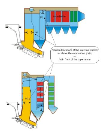
Figure 5-39 Schematic of WTE unit with proposed locations of injection system [41]
