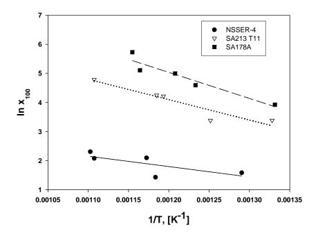
Figure 5-4 Temperature dependence of penetrations of three different materials (SA178A, SA213T11, and NSSER-4) after the 100-hour test
