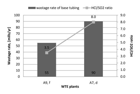
Figure 3-10 Wastage rates of waterwall base tubing and HCI/SO<sub>2</sub> ratio
