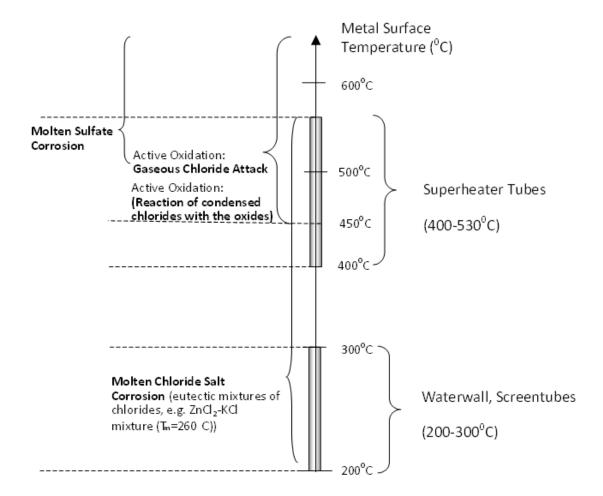
Figure 2-1 Schematic on the influence of temperature on different corrosion mechanisms on boiler tubes [7]
