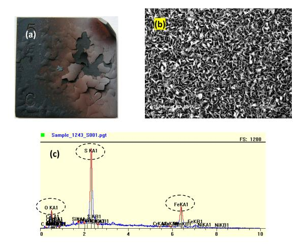
Figure 5-18 (a) Surface morphology of sample SA178A tested with 1000ppm HCl-containing gases, (b) SEM images of the scale, and (c) Elemental analysis of the scale
