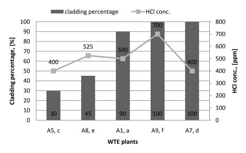
Figure 3-3 Waterwall cladding percentage and HCl conc. in process gas
