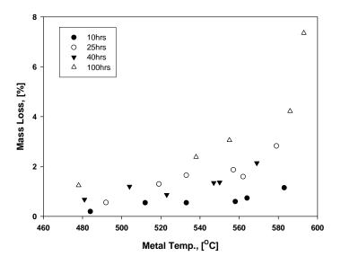
Figure 5-1 Effect of metal temperature on mass loss of samples
