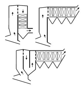
Figure 2-2 Schematic diagram of vertical and horizontal boilers [10]
