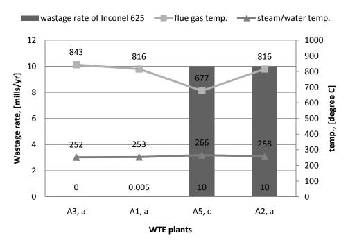
Figure 3-12 Wastage rates of Inconel 625, flue gas, and steam/water temperatures
