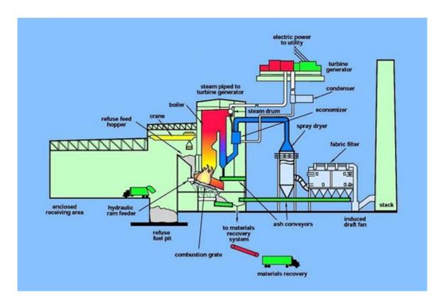
Figure 1-1 Schematic diagram of a typical waste-to-energy facility [2]
