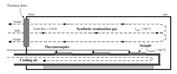
Figure 4-3 The schematic cross-section of the furnace and sample carrier
