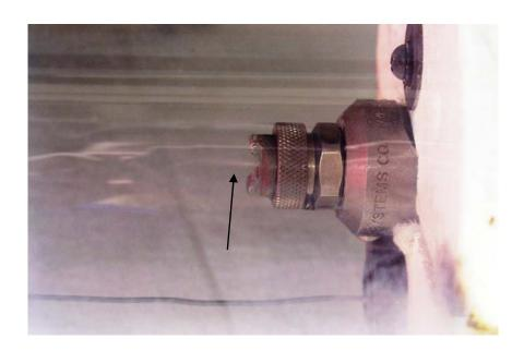
Figure 4-9 The spray pattern generated with air and fluid pressure at 3 and 2 psi, respectively
