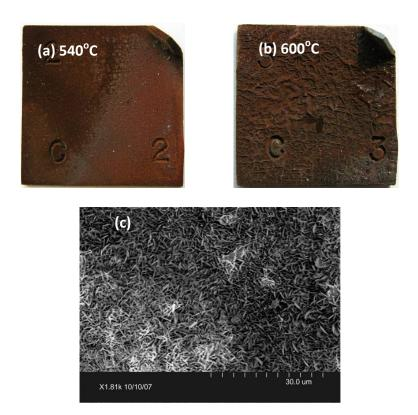
Figure 5-11 Surface morphologies of samples of alloy SA178A after the 100-hour test
