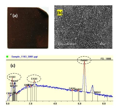
Figure 5-15 (a) Surface morphology of sample SA178A tested at 560°C metal temperature with non HCl-containing gases, (b) SEM images of the scale, and (c) Elemental analysis of the scale
