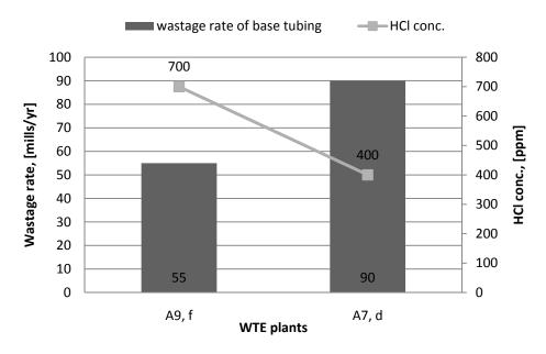
Figure 3-7 Wastage rates of waterwall base tubing and HCl conc. in process gas
