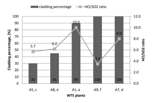
Figure 3-5 Waterwall cladding percentage and HCl/SO<sub>2</sub> ratio
