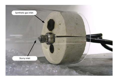
Figure 4-8 The configuration of the nozzle and synthetic gas inlet
