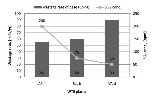
Figure 3-9 Wastage rates of waterwall base tubing and SO<sub>2</sub> conc. in process gas
