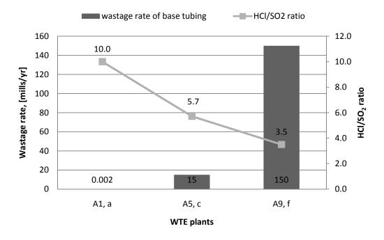
Figure 3-16 Wastage rates of superheater base tubing and HCI/SO<sub>2</sub> ratio
