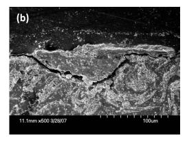
Figure 5-8 Cross-sectional SEM images of the remaining sample substrates: (a) metal temperatures = 630°C and (b) metal temperatures = 502°C
