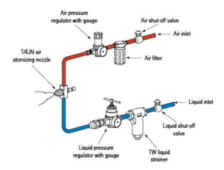
Figure 4-7 The schematic of the injection system [34]
