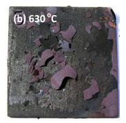
Figure 5-9 Surface morphologies of samples of SA213 T11 after the 100-hour test
