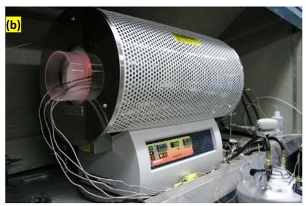
Figure 4-6 Configuration of the tube furnace and injection system; (a) seen from the right side and (b) seen from the left side of the furnace
