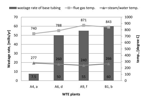
Figure 3-13 Wastage rates of waterwall base tubing, flue gas, and steam/water temperatures
