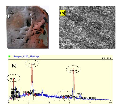
Figure 5-26 (a) Surface morphology of sample SA213 T11 tested at metal temperature of 565°C with 1000ppm HCl-containing gases, (b) SEM images of the scale, and (c)
