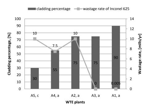
Figure 3-1 Waterwall cladding percentage and wastage rate of Inconel 625
