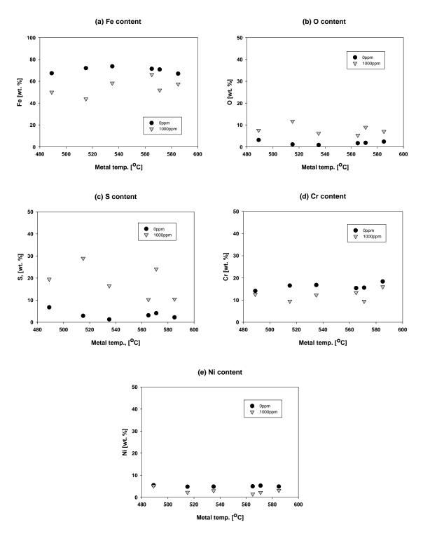
Figure 5-36 Elemental analysis of the scales' surfaces; (a) Fe, (b) O, (c) S, (d) Cr, and (e) Ni
