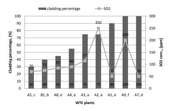
Figure 3-4 Waterwall cladding percentage and SO<sub>2</sub> conc. in process gas
