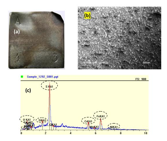
Figure 5-33 (a) Surface morphology of sample NSSER-4 tested with 1000ppm HCl-containing gases, (b) SEM images of the scale, and (c) Elemental analysis of the scale
