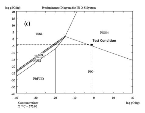
Figure 5-32 Stability diagrams of the system at  $575^{\circ}$ C (without HCl) (a) Fe-O<sub>2</sub>- SO<sub>2</sub>, (b) Cr-O<sub>2</sub>-SO<sub>2</sub>, and (c) Ni-O<sub>2</sub>-SO<sub>2</sub>
