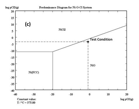
Figure 5-34 Stability diagrams of the system at  $575^{\circ}$ C (with 1000ppm HCl) (a) Fe-O<sub>2</sub>-Cl<sub>2</sub>, (b) Cr-O<sub>2</sub>-Cl<sub>2</sub>, and (c) Ni-O<sub>2</sub>-Cl<sub>2</sub>
