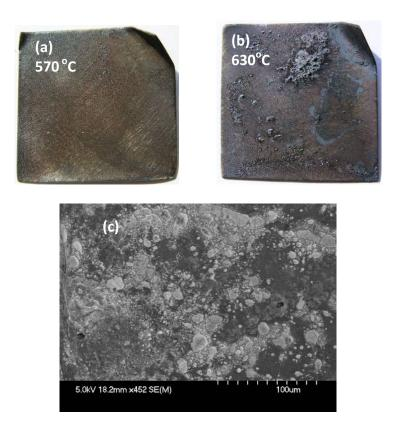
Figure 5-5 Surface morphologies of two samples of NSSER-4 at different metal temperatures after 100-hour test
