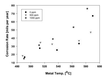
Figure 5-30 Comparison of mass loss corrosion rates
