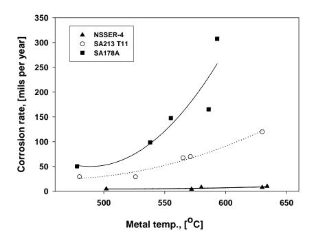
Figure 5-13 Comparison of mass loss corrosion rate
