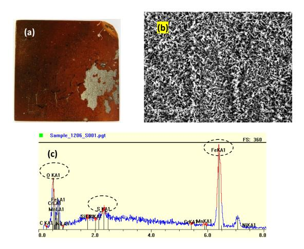
Figure 5-23 (a) Surface morphology of sample SA213 T11 tested at metal temperature of 570°C with non HCl-containing gases, (b) SEM images of the scale, and (c) Elemental analysis of the scale
