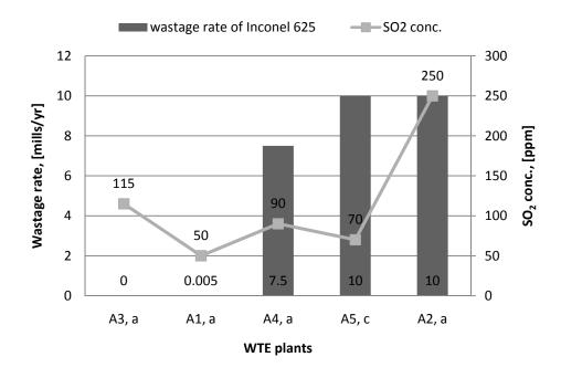
Figure 3-8 Wastage rates of Inconel 625 and SO<sub>2</sub> conc. in process gas
