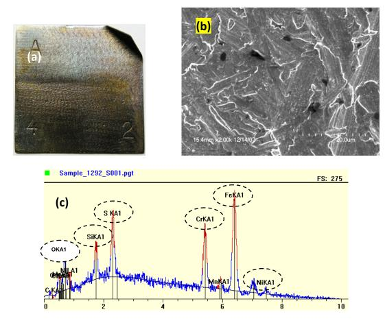
Figure 5-31 (a) Surface morphology of sample NSSER-4 tested at metal temperature of  $575^{\circ}$ C with non HCl-containing gases, (b) SEM images of the scale, and (c) Elemental analysis of the scale
