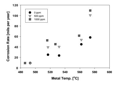
Figure 5-22 Comparison of mass loss corrosion rates
