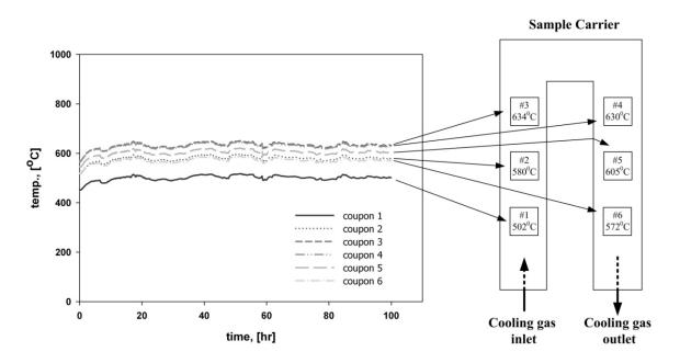
Figure 4-4 Temperature profiles of six samples on carrier
