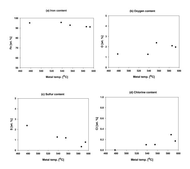
Figure 5-12 Elemental analysis of surfaces of alloy SA178A: (a) Fe, (b) O, (c) S, and (d) Cl
