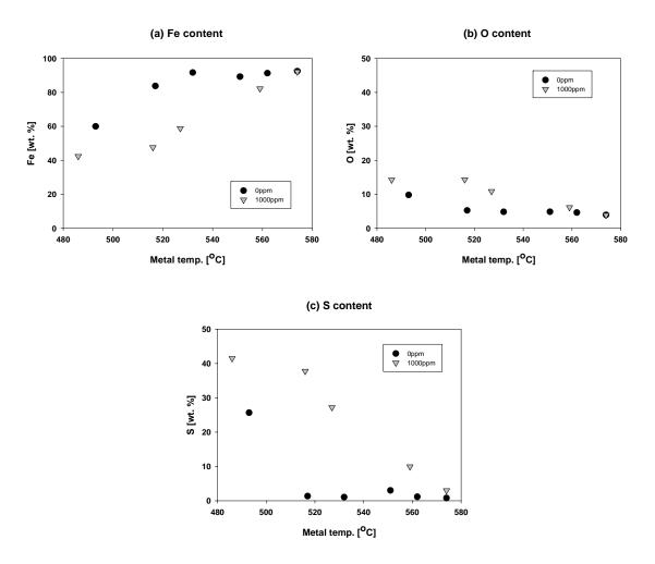
Figure 5-21 Elemental analysis of the scales' surfaces; (a) Fe, (b) O, and (c) S
