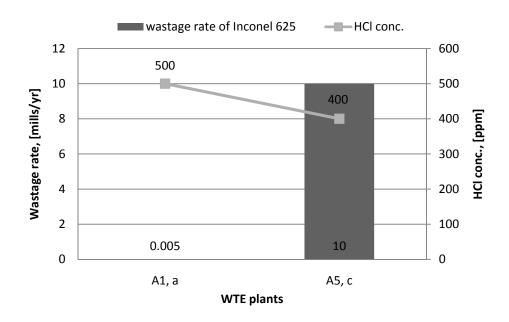
Figure 3-6 Wastage rates of Inconel 625 and HCl conc. in process gas
