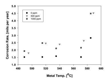
Figure 5-37 Comparison of mass loss corrosion rates
