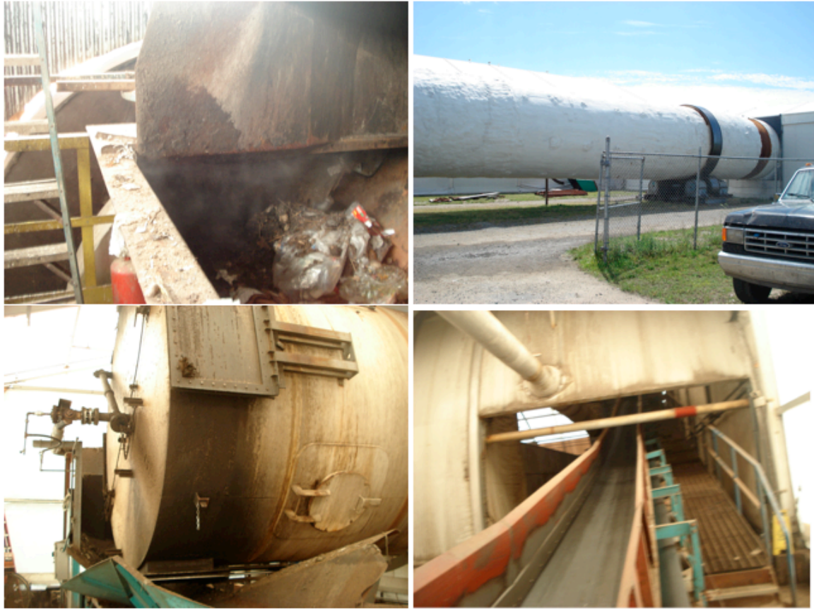
Figure 20 a,b,c,d. a: mixed waste entering the rotating drum. b: Outside view of the rotating drum. c: End piece of the drum where the unstabilized material is falls out of the device. d: Conveyor belt that transports the waste to an area where it is windrowed and aerated for curing.
