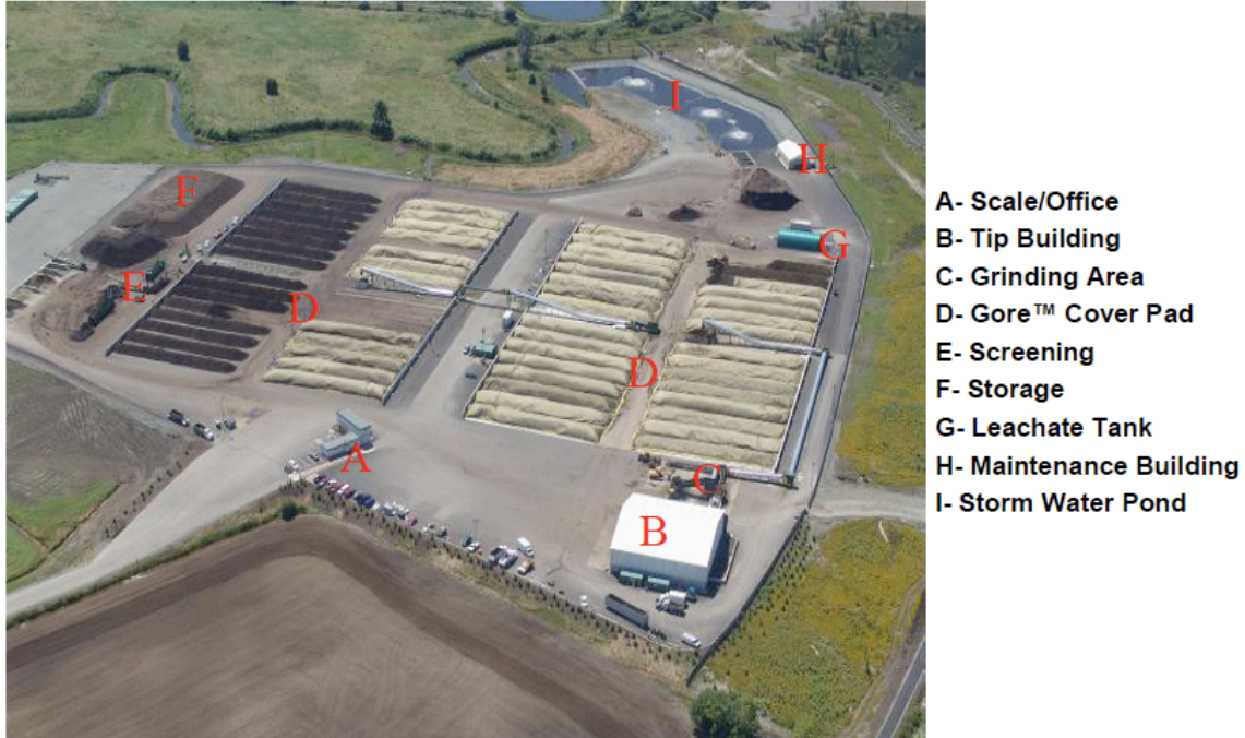
Figure 9: Aerial view of the Gore covered composting site in Cedar Grove, Seattle.
