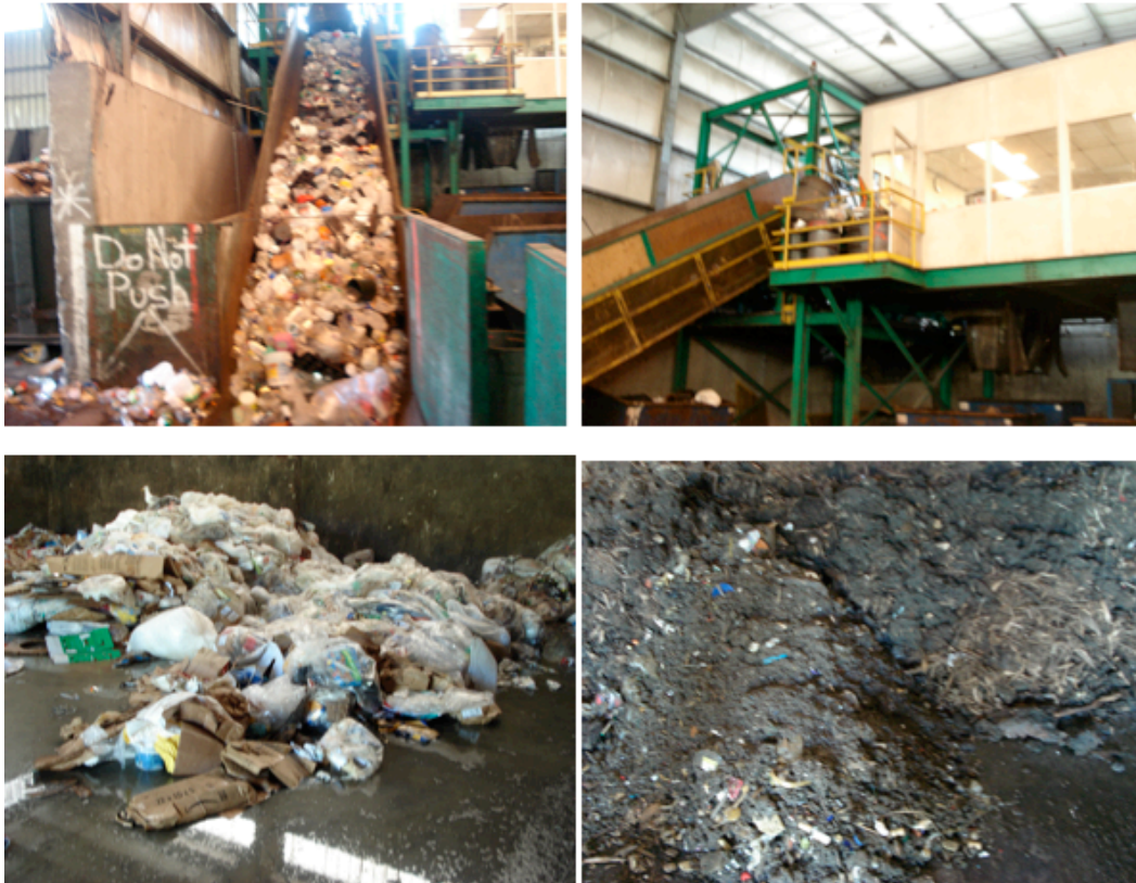
Figure 18 a,b,c,d. a: Plastic pushed onto a conveyor belt and separation of metals by magnet at the end. b: Place where the plastic stream enters the picking room. c: Temporary storage of contaminated plastics that are separated out of the plastic stream. I also spotted some cardboard and paper. This is later mixed in with the organic waste that enters the rotary drum digester. d: Sludge from a Wisconsin WWTP that is also mixed in with the rotary digester.
