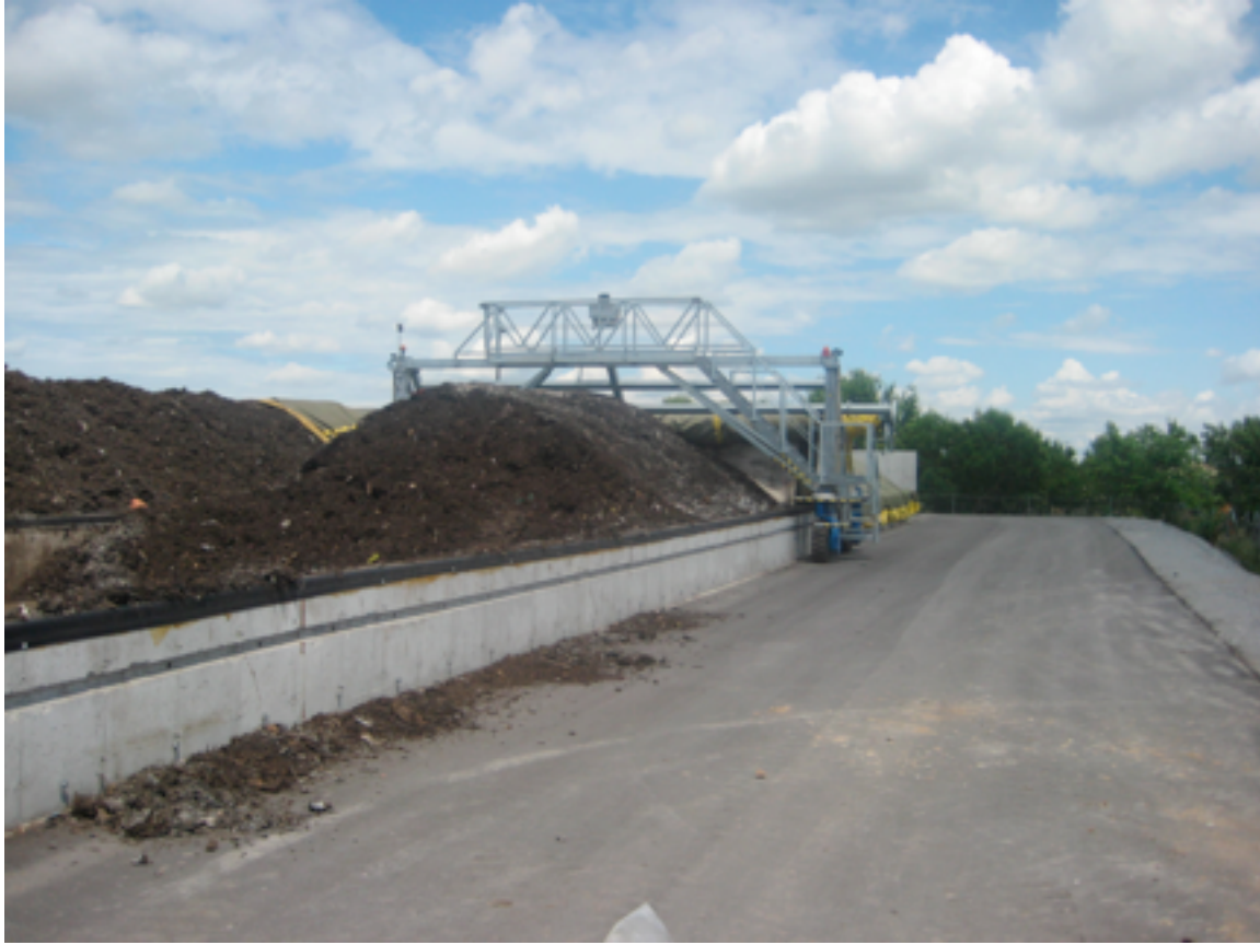
Figure 15: Winding machine at the Walker compost facility. Sensors on the sides keep the machine from hitting the walls and make it possible to be operated by one person. The Gore membrane cloth is simply rolled off the machine to cover the pile. The sides are secured to the wall with rubber ropes.
