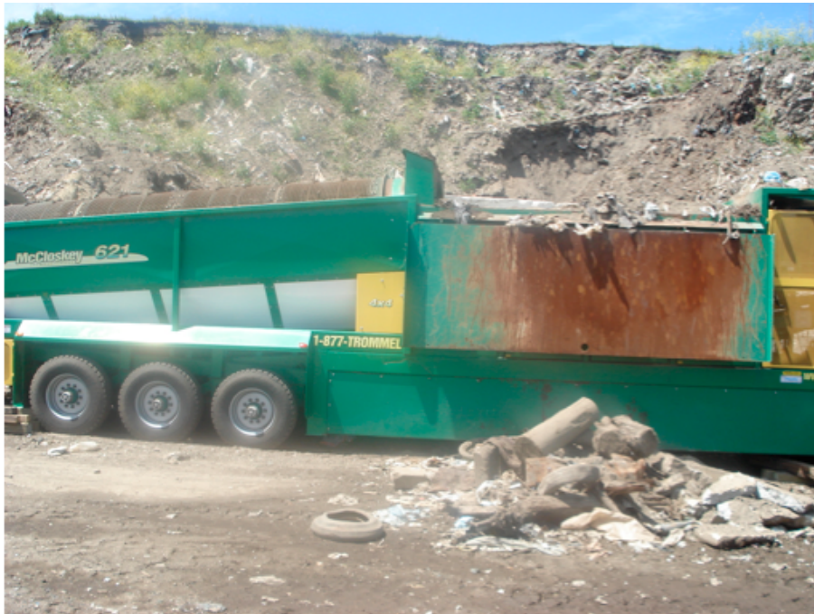
Figure 23: A McCloskey 621 Trommel device separating bulky waste (in foreground). This device is used for the mining of the old landfill.
