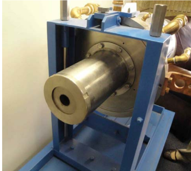
Figure 43. Exit nozzle of Marc 11 Plasma torch (six Marc 11 torches will be required for a 750 tons/day plant)
