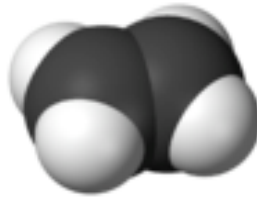
Figure 2.5 : Ethylene C_2H_4 monomer, the basis for polyethylene
