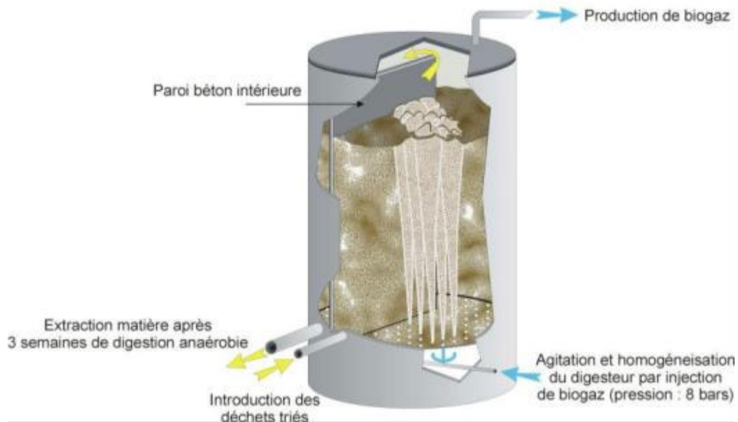
Figure 10 Valorga AD reactor
