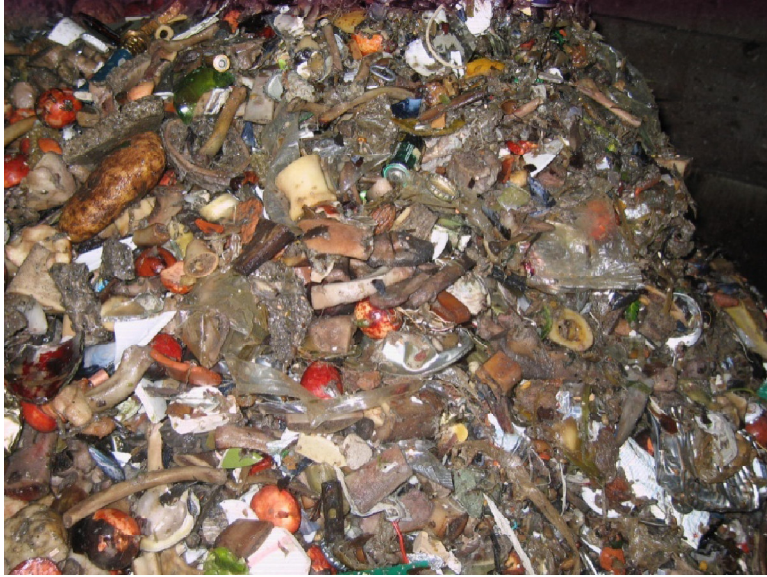
Figure 17 Floating and heavy fractions separated at Dufferin AD facility (photo by L. Arsova)
