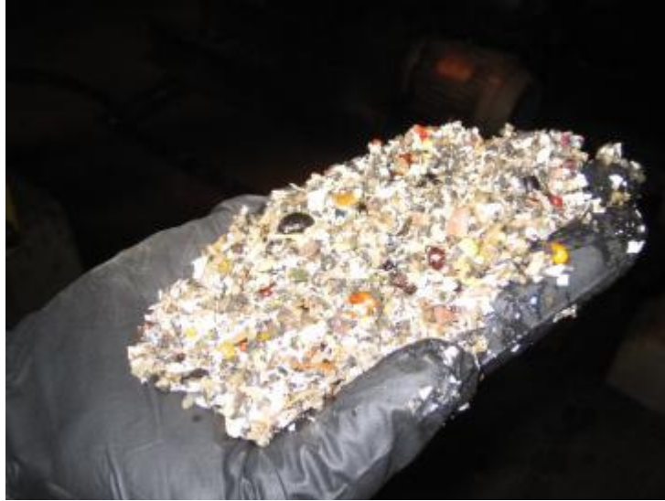
Figure 16 Grit fraction at Dufferin AD plant (photo by L. Arsova)
