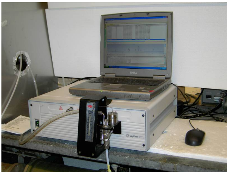
Fig. 3.10. Agilent 3000 Micro GC and notebook computer to acquire gas chromatograph data.
