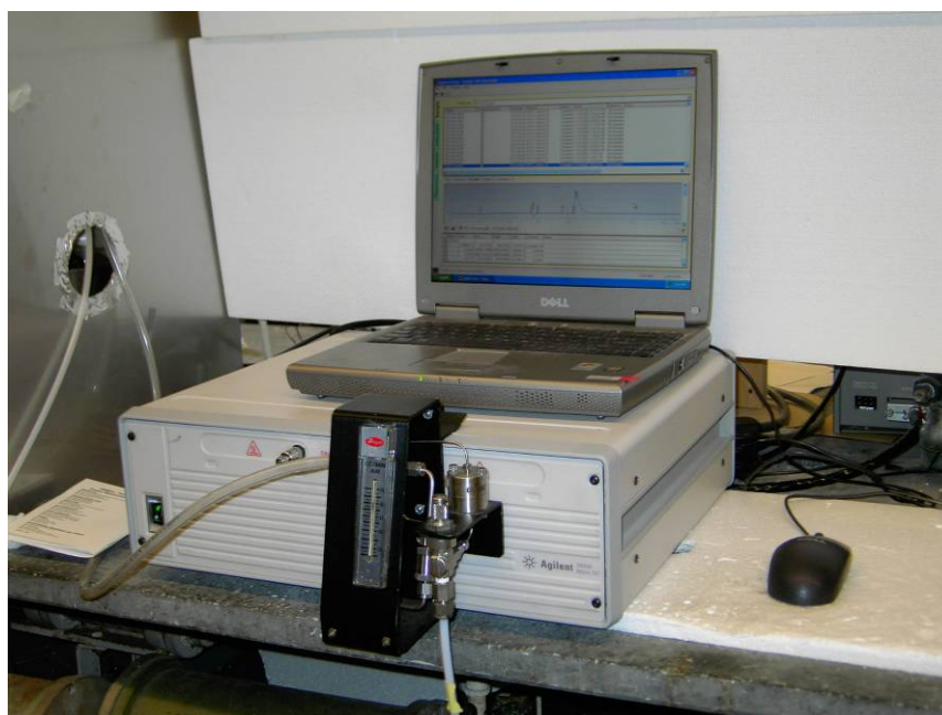
Figure 4: Agilent 3000 Micro GC and notebook computer to acquire gas chromatograph data.
