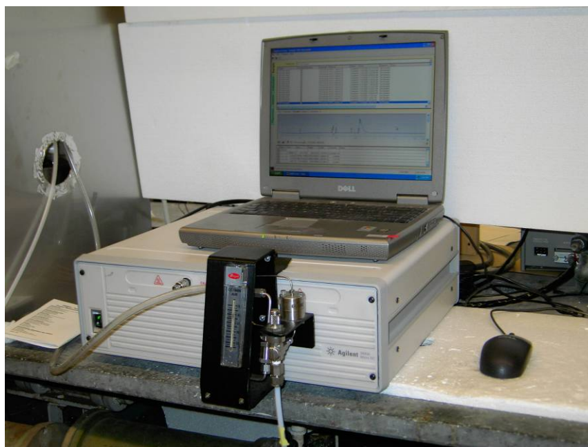
Figure 4: Agilent 3000 Micro GC and notebook computer to acquire gas chromatograph data.
