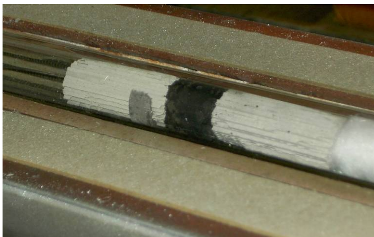
Fig 5.19. Nickel catalyst following stoichiometric reforming studies. The catalyst began as spherical pellets, but became encrusted by solid carbon buildup.
