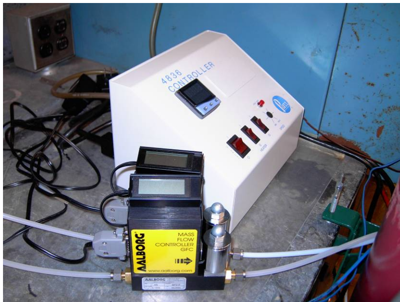
Figure 3: Parr Instruments 4835 temperature controller and Aalborg GFC17 mass flow controllers.
