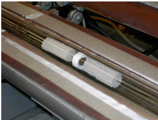
Fig 3.7. Reactor shown with blank monoliths holding thermocouples on either end of the Rh monolith, wrapped with insulating material.
