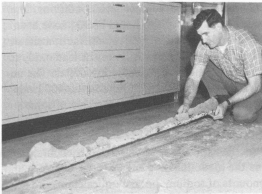
FIG. 1 DEPOSIT ACCUMULATED ON PROBE IN MIAMI COUNTY, OHIO, INCINERATOR AFTER 828 hr
