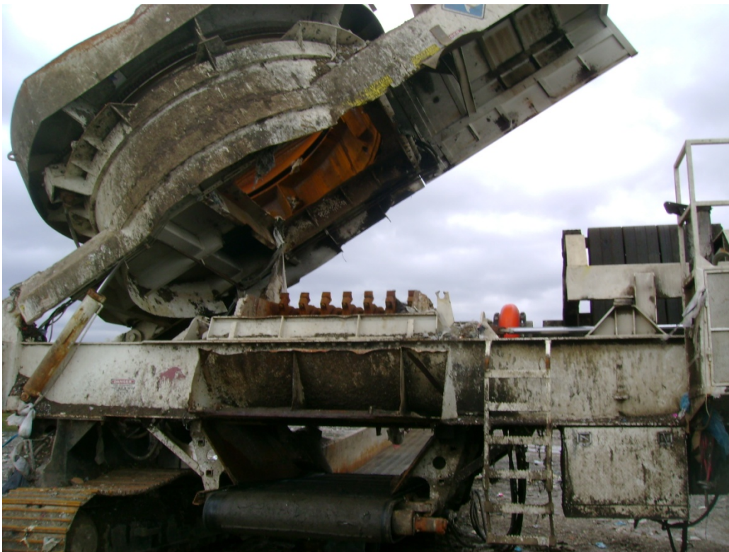
Figure 30: SWG 1600 hammermill used at Albany city landfill.
