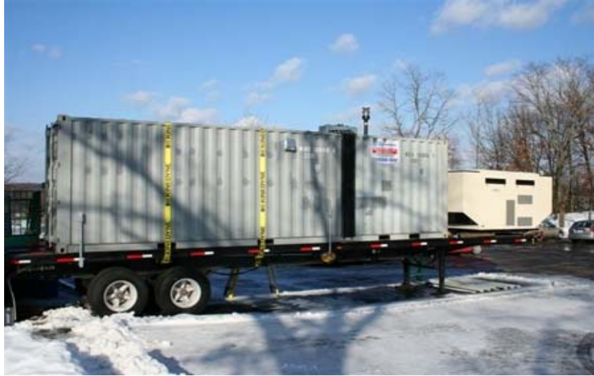
Figure 14 Energy's Mobile GEM 3T120 Gasification System 41
