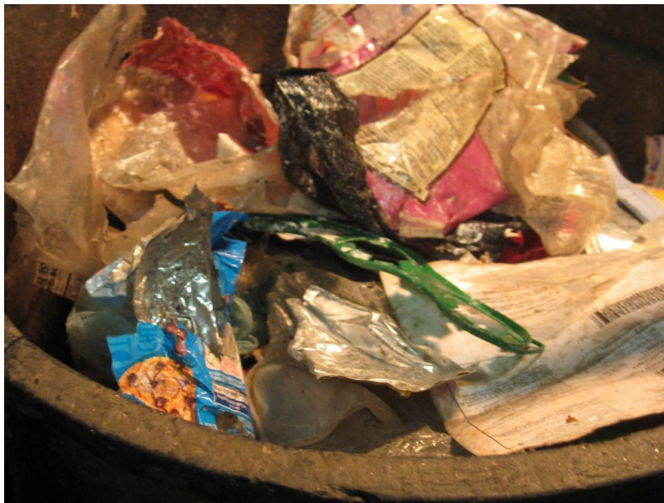
Manually Separated Plastic Film Residue
