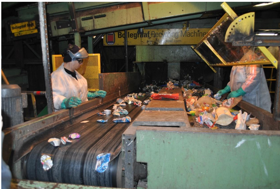
Separation stations for metal cans and mixed plastic
