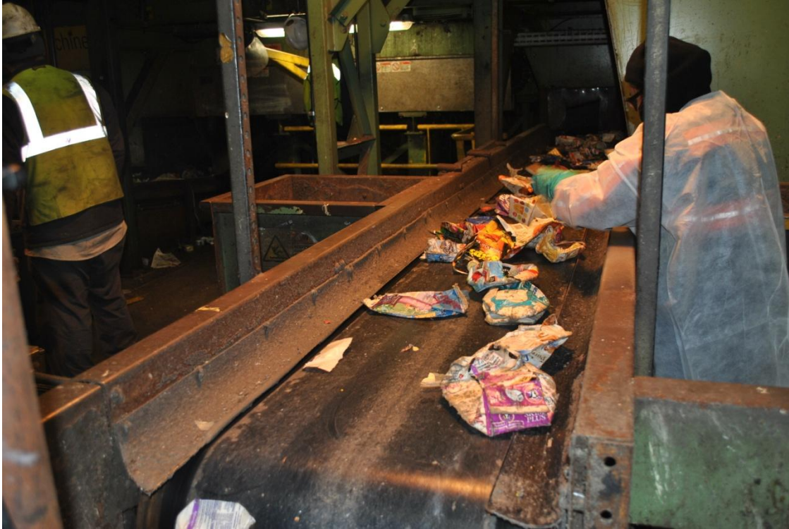
Aseptic cartons separation line
