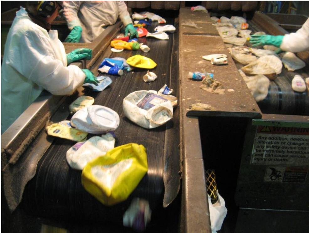
Separation lines for colored and natural HDPE
