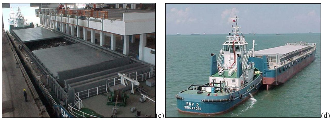
Figure 6.6 Loading waste on barge with built-in containers (171) .
