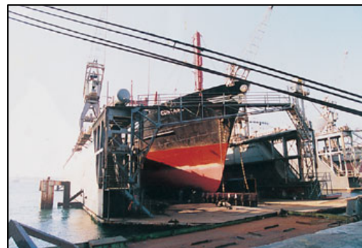
Figure 3.55 Floating dock of the ship repair zone (166) .
