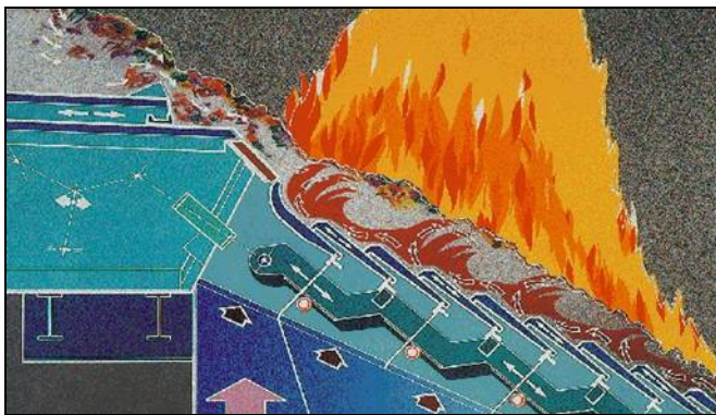
Figure 2.13 Motion of the grate bars (156) .
