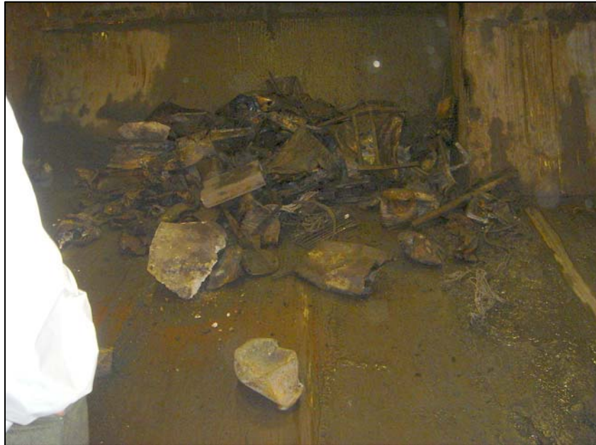
Figure 5.15 Materials extracted from ash by grizzly – Veolia ES (Montenay) Dutchess LLC WTE facility at Poughkeepsie, NY, USA.
