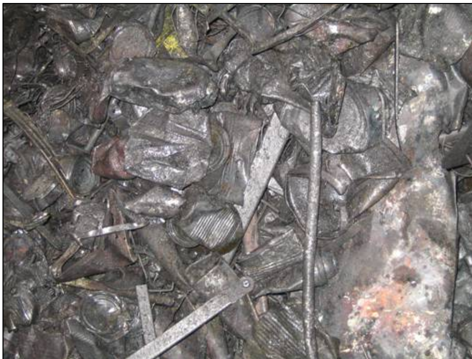
Figure 5.17 Ferrous metal fraction after magnetic separation – Veolia ES (Montenay) Dutchess LLC WTE facility at Poughkeepsie, NY, USA (54) .
