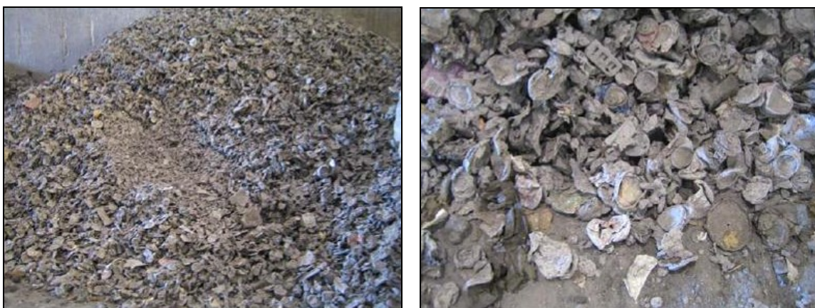
Figure 5.18 Extracted non-ferrous metal fraction – Resource Recovery, LLC, Pinellas Facility at St. Petersburg, FL, USA (53) .
