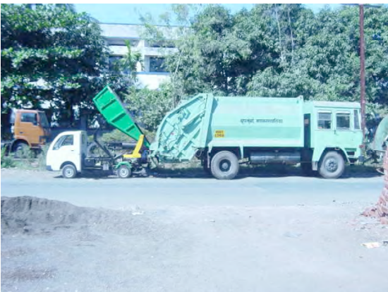
Figure 26c: One-ton vehicle unloading MSW into large compactor {9}
