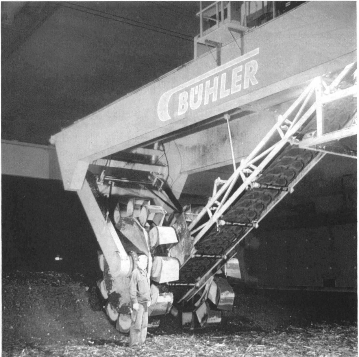
FIG. 5(b) WENDELIN™ TURNER IN COMPOSTING BUILDING
