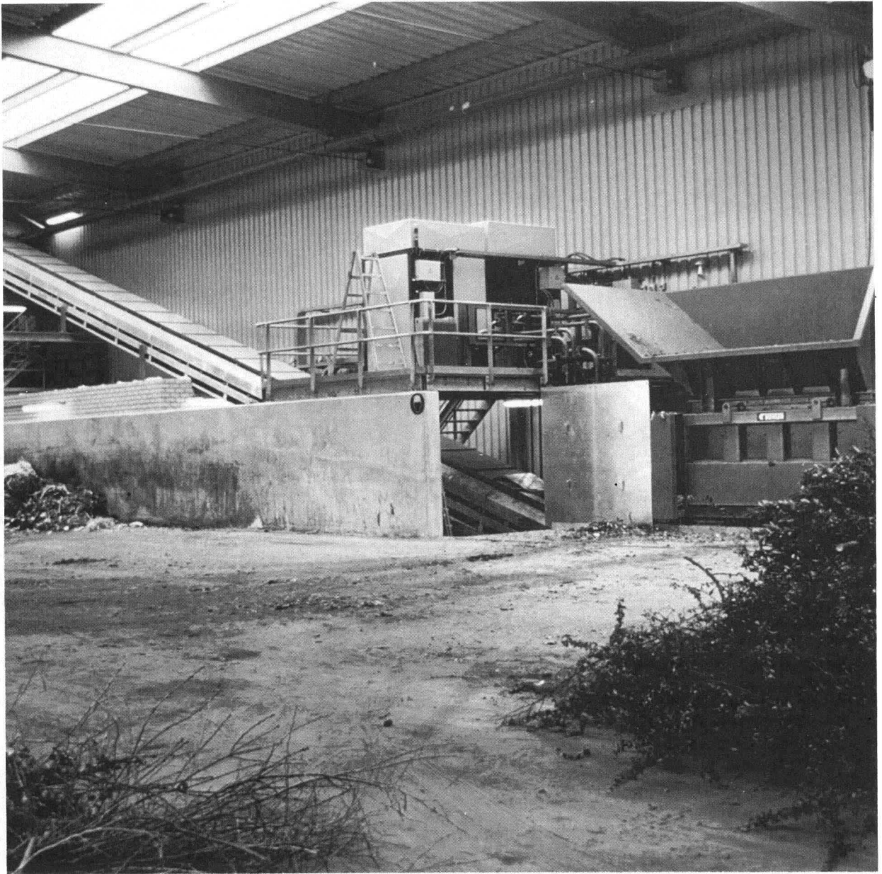
FIG. 5(a) TIP FLOOR WITH TRIMALIN™ SHREDDER AND BELT CONVEYOR TO SCREENING DRUM
