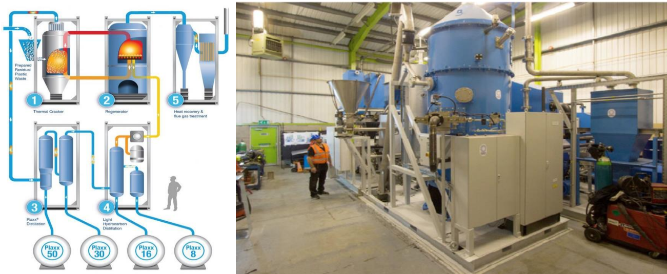
Fig. 4 Schematic diagram of the technical process and the commercial-scale unit of Recycling Technologies
