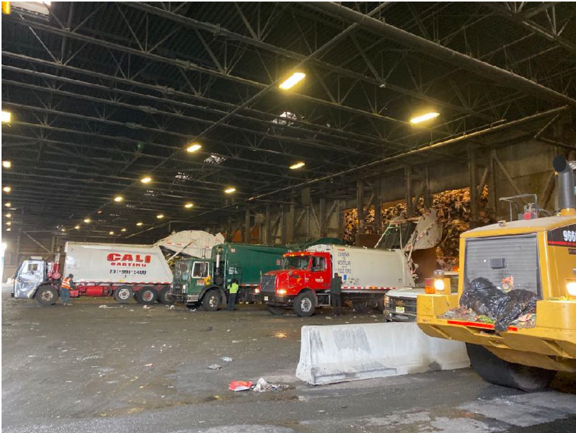
Figure 3: Municipal waste is delivered to the facility and stored in a bunker. It's closed for delivery on Sundays, where they use up the waste stock. In addition to Municipal Waste, Covanta is allowed to receive commercial and industrial waste, but receives mostly MSW.
