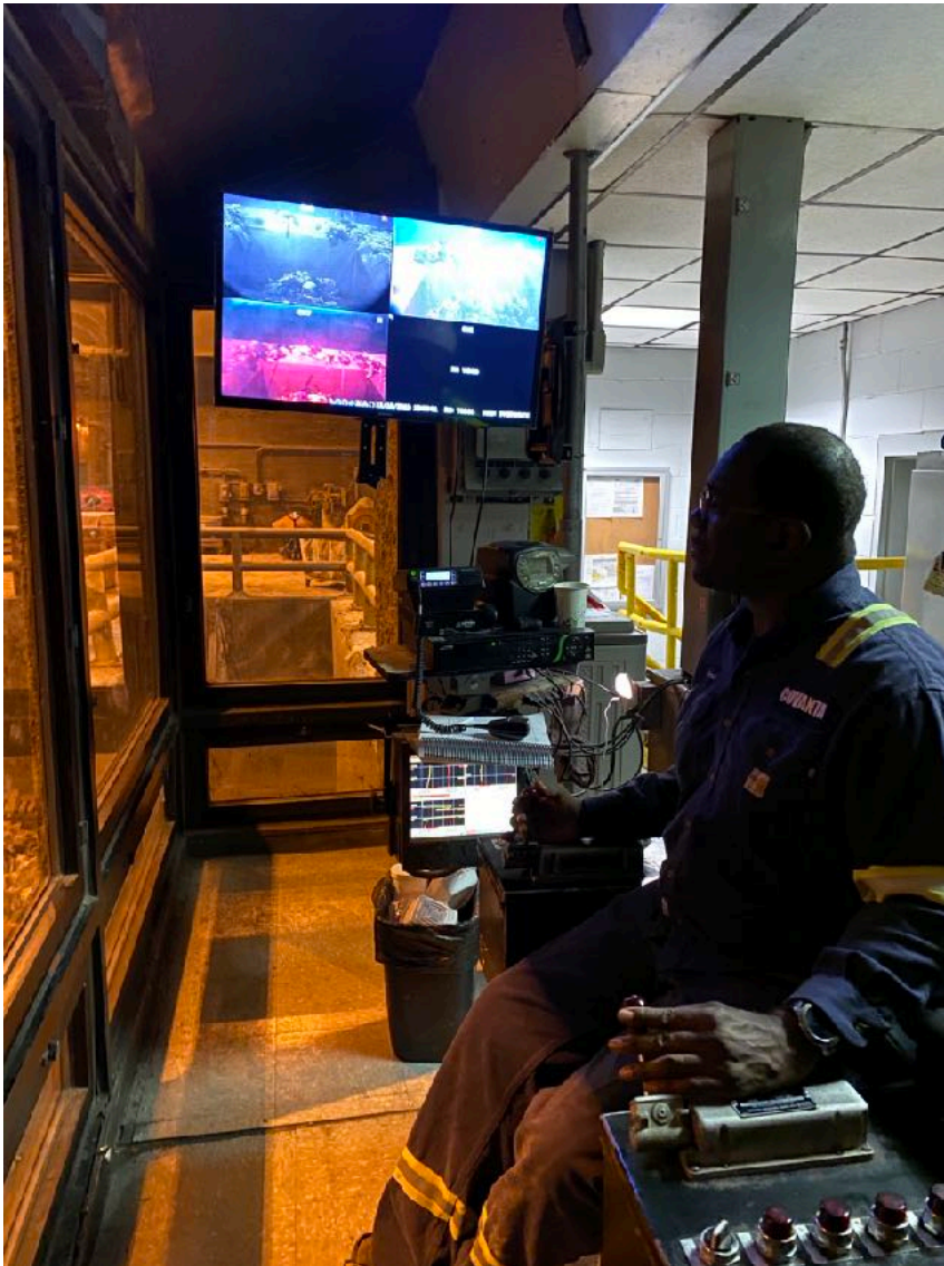
Figure 5: Crane operator, who is responsible for managing waste inside the waste bunker and feeding the boilers.
