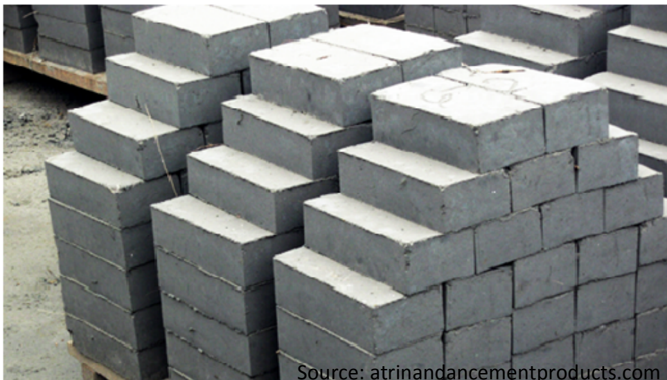
Figure 7 Fly ash and bottom ash can be reused if treated properly. The ash is used to make construction materials, such as bricks and concrete.
